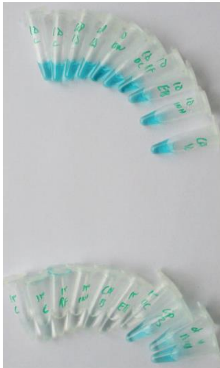
FIG. 1. In response to bacterial growth, the malachite green indicator changes in color from green to the total loss of color.
